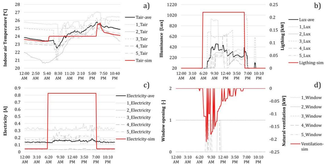
Figure 6. Occupants' behavior simulation (red lines) results vs. monitored data in terms of a) indoor air temperature, b) illuminance over the working plane, c) equipment electricity consumption, and d) windows opening.
