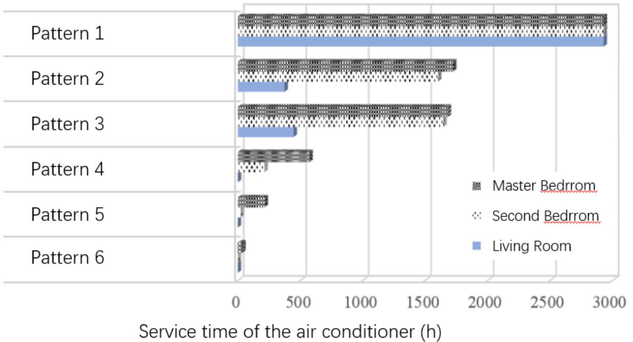
The figure above shows the service time of the air conditioner. It can be seen that the service time under pattern 1 could be about 3000 hours, while pattern 2 and pattern 3 is 1700h, which is half of pattern 1. And the pattern 4 \5\6 only use the AC for 600h\200h\40h.
