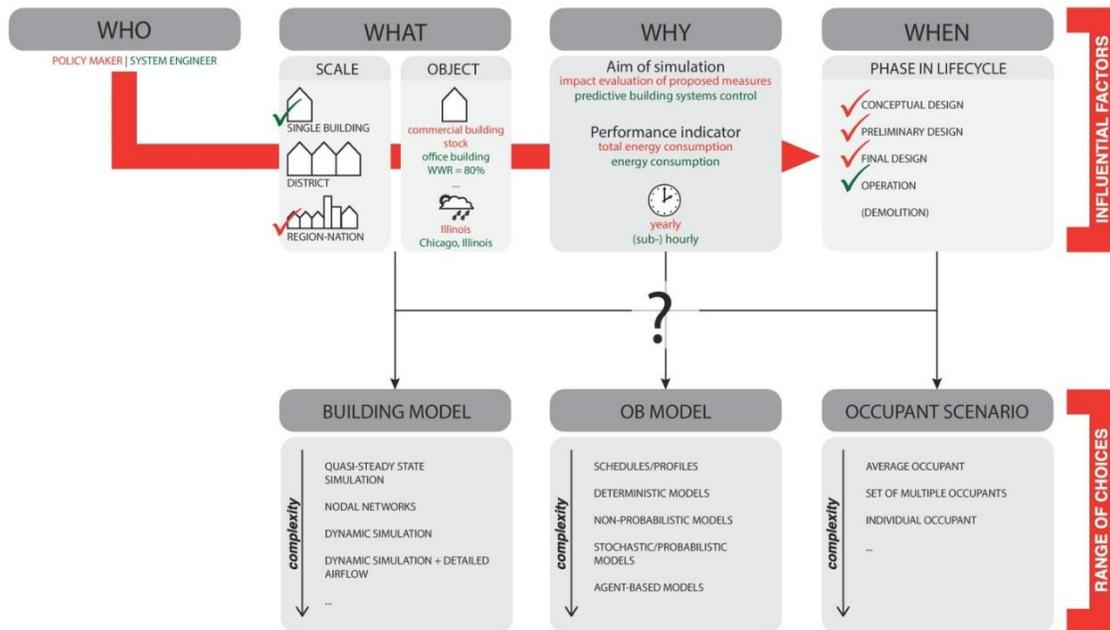
Figure 1: Graphical presentation of the driving factors (who, what, why, when) upon which a suitable energy modeling technique should be elaborated for each specific case (Gaetani, Hoes, and Hensen 2016).
